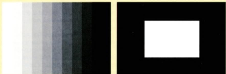
Left, the vertical grayscale pattern from Ovation Software's *Avia* home theater test/setup DVD, ranging from peak white to black, is used to visually evaluate a TV set's grayscale tracking. Right, the high-level (100-IRE) window test pattern from the *Avia* disc is used to measure both color temperature and brightness.
